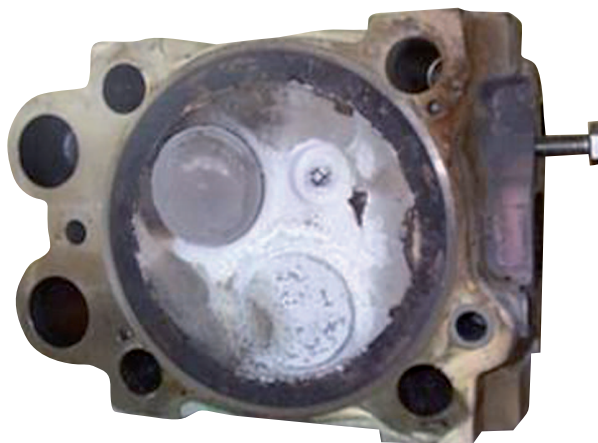
Silica deposits on a head & valves causing a collision between valves and piston crown
