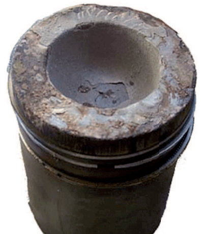
A piston coated in silica deposits
